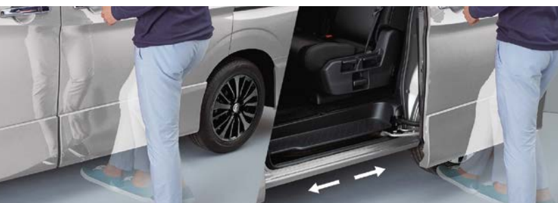
HANDS-FREE DUAL POWER SLIDING DOORS opening the door with just your feet while hands are full.
